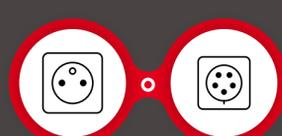
Electric trucks from Renault Trucks can be recharged very simply using a regular AC outlet (for the Renault Trucks Master) or a three-phase industrial socket (for D and D Wide trucks). It takes between 6 and 12 hours.
